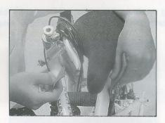
3. Placing your right hand on the seat tube and your left hand on the front fork, gently unfold and straighten the MTB.
