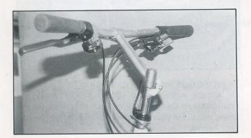
The second way is just to raise or lower the handlebar expansion arm. Loosen the handle stem clamp with an Allen wrench, and raise or lower the handlebar. Don't forget to tighten the clamp afterward.
