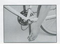
6. Loosen the seat post pillar pin bolt. Raise the seat post to the desired level and tighten the pillar pin bolt. (CAUTION: Do not raise the seat post past the "SAFETY MARK" on the back of the seat post.)
