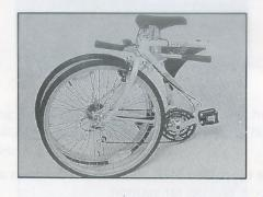
2. Loosen and remove the Velcro tape wrapping from between the seat tube and front top tube.
