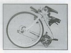
2. Loosen and remove the Velcro tape wrapping from between the seat tube and the front top tube.
