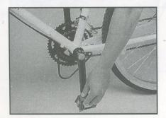
6. Using the 6mm Allen wrench, loosen the frame lug lock bolts. (NOTE: Do not loosen the bolts completely).
