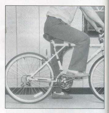
To get the right height, ask someone to hold your bicycle upright while you sit on the saddle. Move the crankshaft so that the ball of your foot rests on the lower pedal. Let your knee bend slightly to get the correct height.
