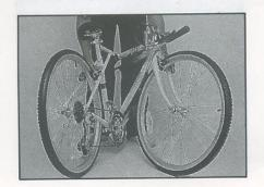
7. Wrap the Velcro strap between the seat tube and the front top tube and strap the MTB folder together.
